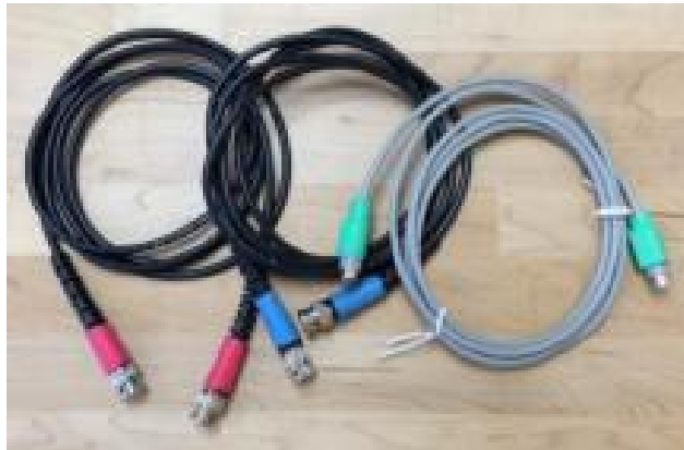
Ref (red) , PC (blue) , Trigger cables (green)
